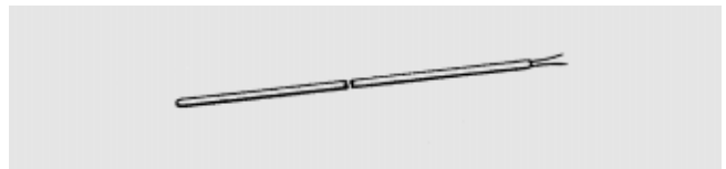
Shielded thermocouple with exposed connecting leads
